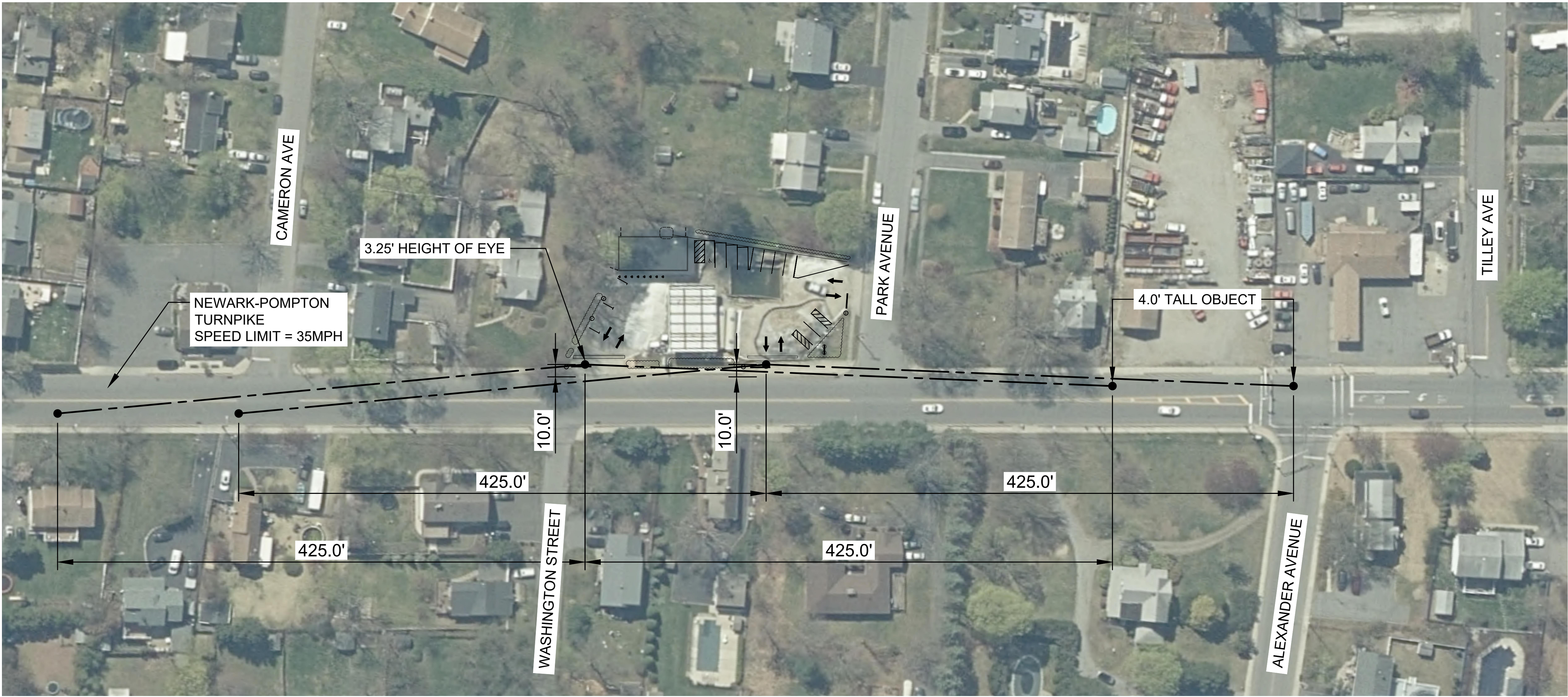
SIGHT DISTANCE EXHIBIT RE: MORRIS COUNTY LAND DEVELOPMENT STANDARDS SECTION 504C, TABLE 500-3 FOR 35 MPH POSTED SPEED LIMIT
